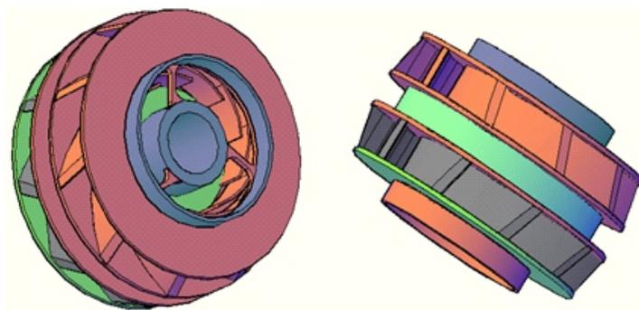
**Figure 3.2: Rotated plain chamfered vane straight impeller**
