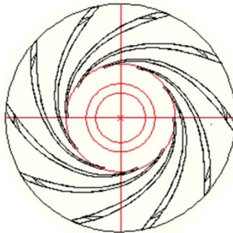
Figure 2.7: Development of Ten Blade 2D Model Impeller
