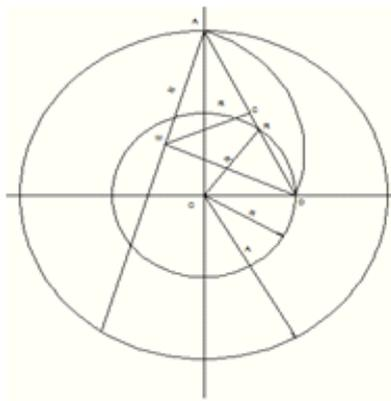
**Figure 1.1: A simple Geometric method of Constructing Vane Profile**
