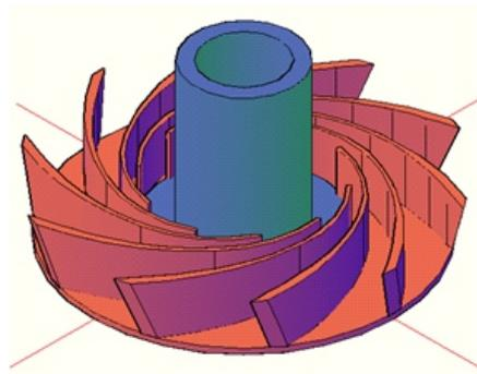
Figure 2.9: Addition of Shaft Sleeve into the vane profile
