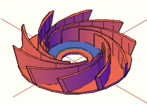
Figure 2.8: Development of Ten Blades 3D Model Impeller
