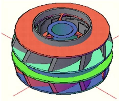
**Figure 2.10: Modeled double-plain vane beveled impeller**
