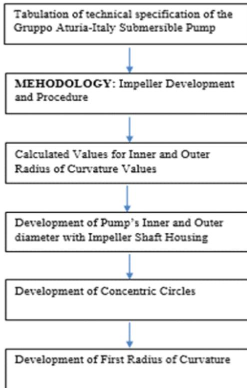
**Figure 2.1: Flow chart for Impeller Development and Modeling**
