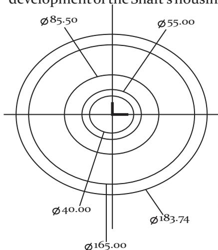
**Figure 2.2: Development of Outer, Inner and Shaft Housing Diameters of the Impeller**
