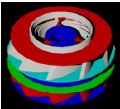
**Figure 3.1: Rendered double-plain vane beveled impeller**
