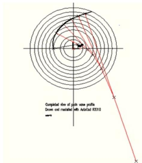
Figure 2.5: Development of the Second Radius of Curvature “EF”
