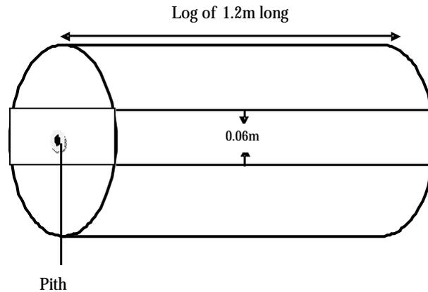
Fig. 2: Diagram of a Billet
