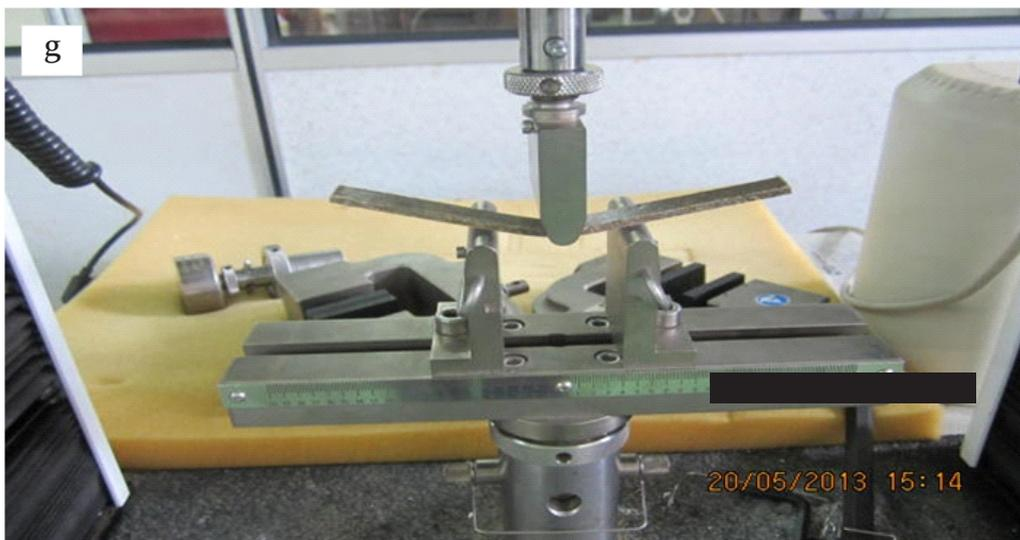
**Figure (g) universal testing of mechanical properties of agro waste composites**
