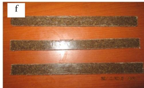
**Figure (f) shows agro waste composite mechanical properties test specimens**
