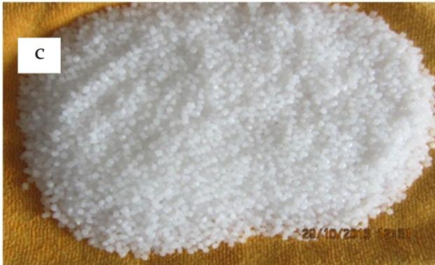
Figure (c) Show High Density Polyethylene (HDPE)
