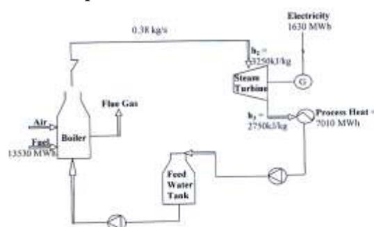
Figure 1: Scenario 1 - Production of electricity and heat from the biomass residues
