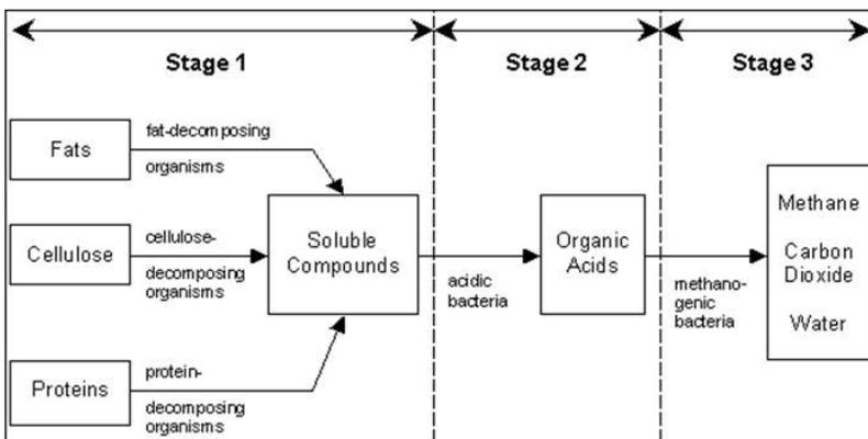
Figure 3: Anaerobic digestion for biogas production.
