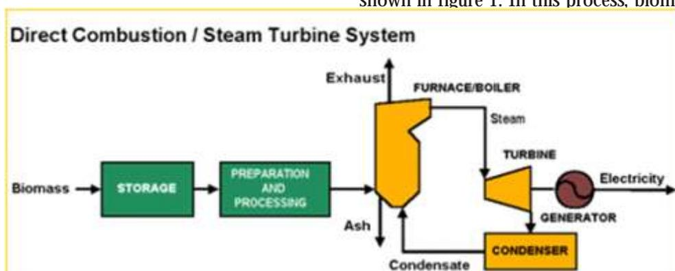
Figure 1: Direct Combustion method of producing Electricity from Biomass
