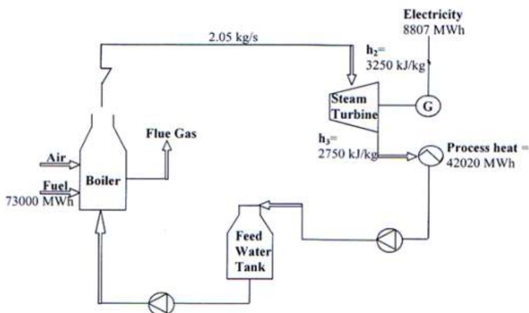
Figure 3: Scenario 2 - Production of Electricity and Heat from Biomass Residues
