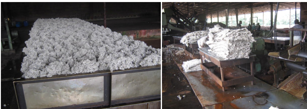
Fig 10: Crumb processing and cleaning
