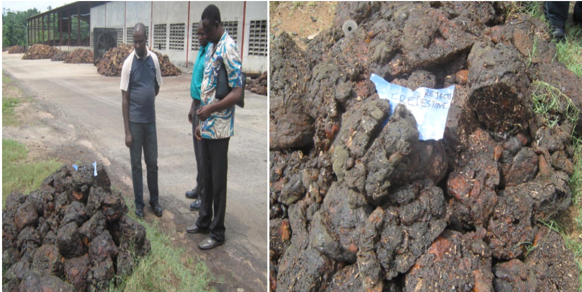
Fig 17: Rejected rubber lump (as a result of deliberate contamination by farmers)
