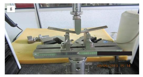
Figure (g) universal testing of mechanical properties of agro waste composites
