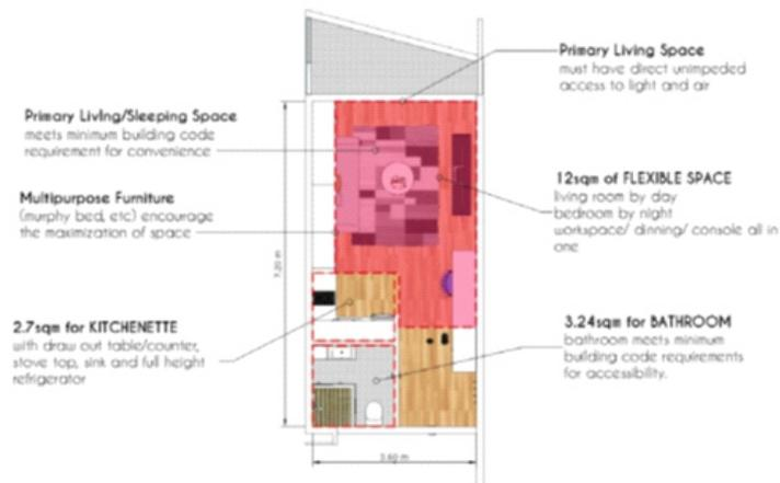
**Figure 6:** Typical floor plan of standard micro unit apartments on Fola Agoro road. (Source: Ogunderu, 2017)
