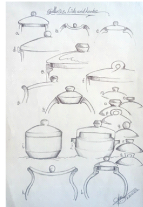
Fig. 8: Drawings to show galleries, lids and knobs
