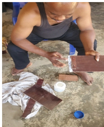
Fig. 6: Applying the White glue for better bonding
