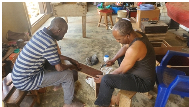
Fig. 7: Nailing the 3 rd side along with the key informant
