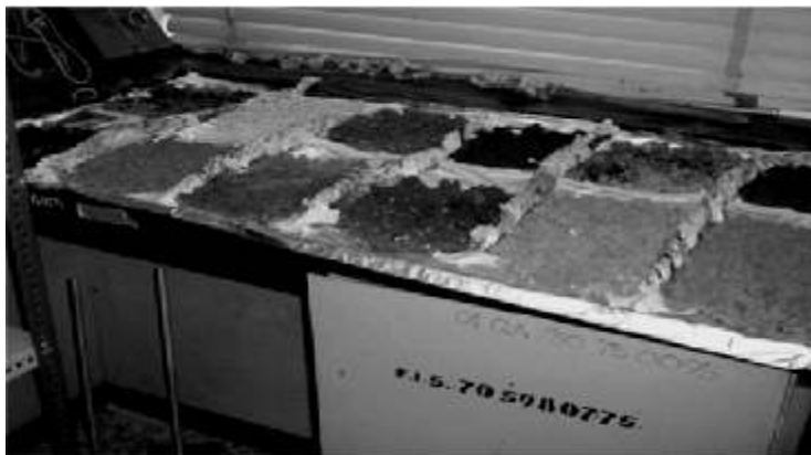
Fig. 2: Sediment variation at different locations of the Lagos lagoon (from top row left are sediment samples from locations A, A2, A3, B, B2 and B3; from bottom row left are C, C2, D, D2, E, and E2 samples)
