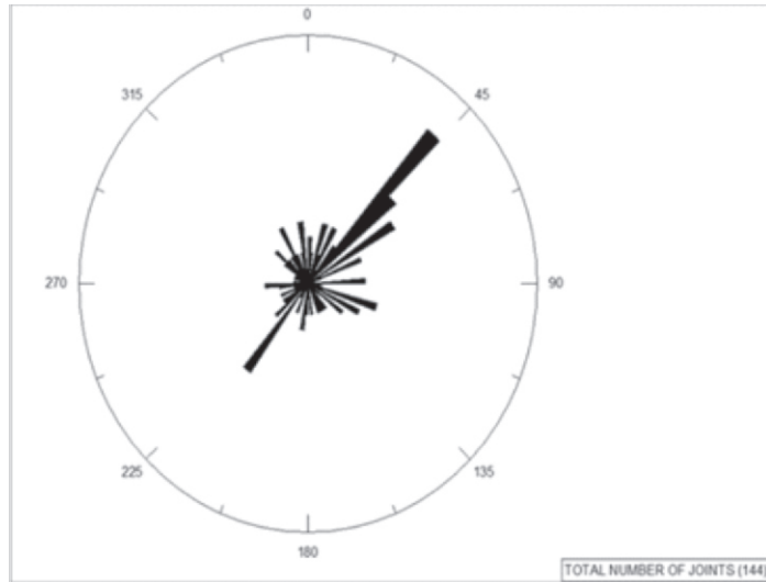
Fig. 8: Rose Diagram of Joints Observed on Quartzite and the Migmatite Rocks in the Study Area
