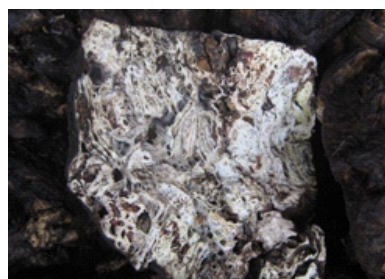
Fig 2: A cut portion of rubber lump to checkmate adulteration
