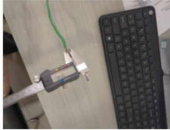
Figure 1: Determining the Diameter of a Wire
