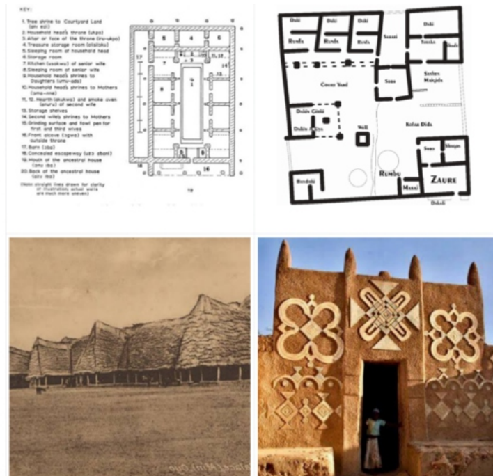
Figure 5: Traditional Ibo homestead layout; traditional Hausa homestead layout, Hausa home façade and decorative motifs; traditional Yoruba elevation. Sources (Clockwise from top left): Henderson & Henderson, (2024); Sa'ad, (1981); Bayt Al Fann, (n.d.), Alaayemoré, (n.d.)
