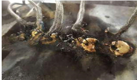
Fig 2: Thermocouple wires connected to the specimen.
