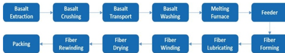
Fig. 2: Flow chart of basalt fiber production
