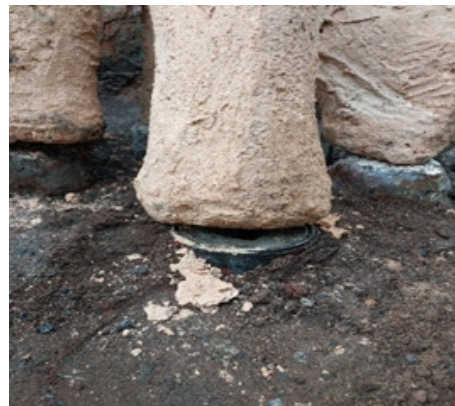
Plate 16: Moulds on the cans ready for dewaxing (stage four).
