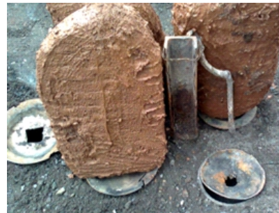
Plate 10: Vertically placed moulds on the metal container for wax collection. Emofonwan's Foundry, Benin May 2020.
