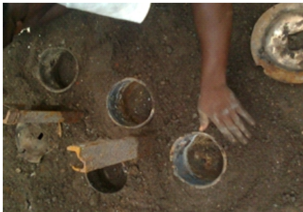
Plate 9: Burying the metal lids for wax collection. Emofonwan's Foundry, Benin city, May 2020.
