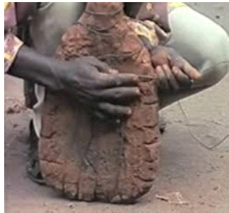
Plate 5: The traditional mould reinforcement, with metal binding wires.
