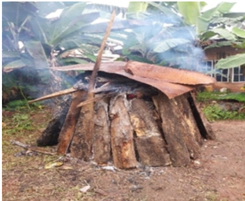
Plate 17: First fire/burning out (stage five) Source: Njk Foundry, May 2024 Benin City
